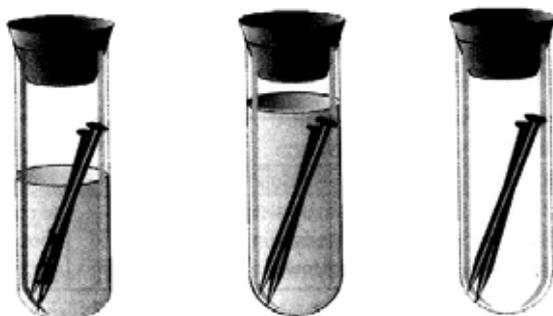
After few days the nails in A are rusted while the nails in B and C are unaffected. Give reasons.
